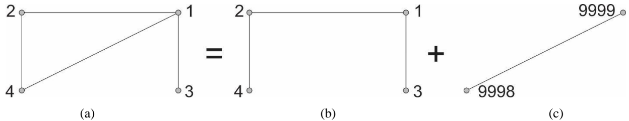
Figure 6. 13: Node Numbering Scheme in the Analytical Models – (a) Standalone Model, (b) Integration Module, and (c) Substructure Module
